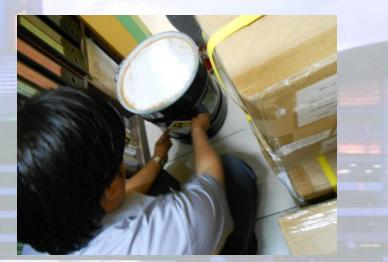
**16.** Affix a leaded tamper proof safety seal onto the shipping drum locking ring and fasten with a hammer or other suitable means.
