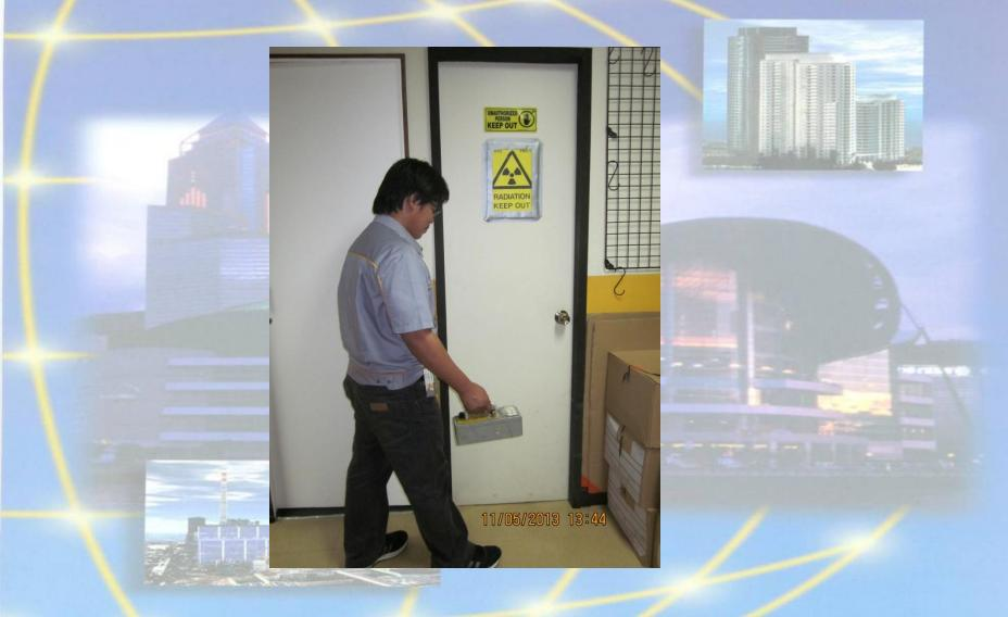
3. If the value is within the allowable, continue approaching the storage area. Survey the outside area of the storage area. The reading shall not exceed 2 mr/hr.
